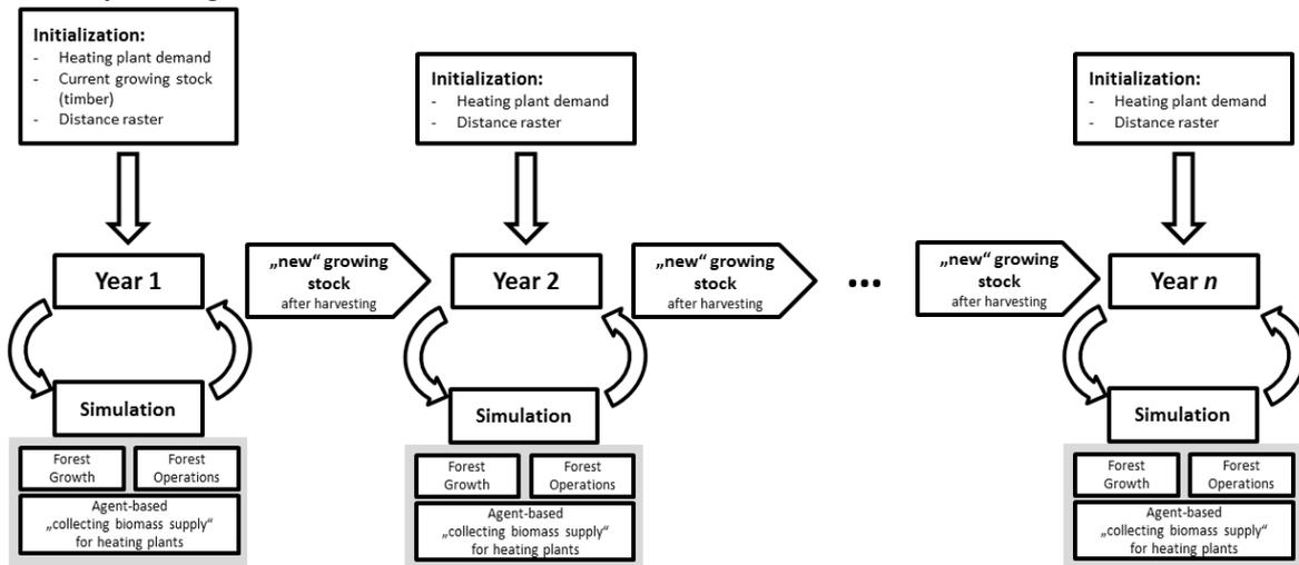
Figure 2. Agent-based simulation approach for each simulation year. This graphic depicts the temporal sequence of the simulation process and the necessary data for each yearly simulation.
