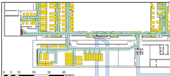
Figure 6: Example showing the graph-based network through the production line environment and possible walking ways as corridors.
