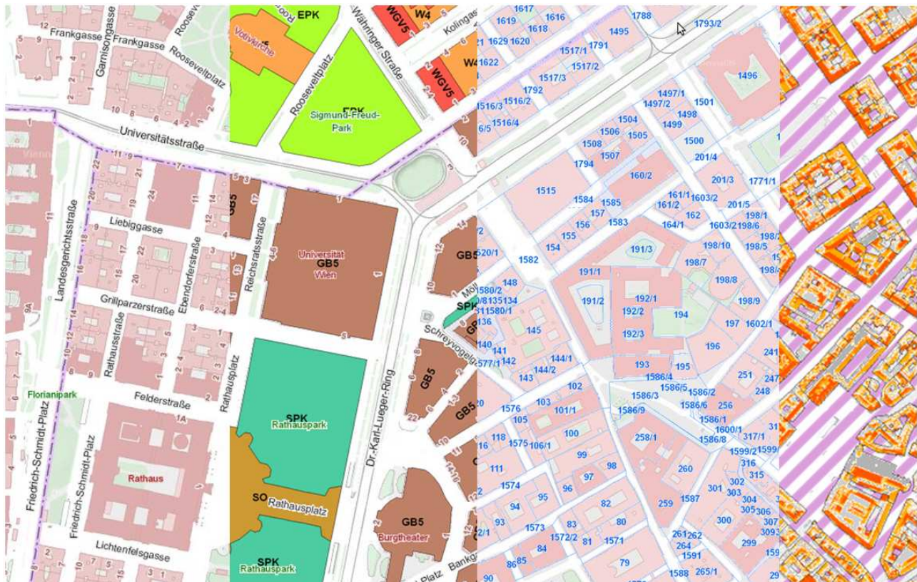
Fig. 1: ViennaGIS maps for the inner city of Vienna showing the Viennese base map (leftmost), land use plan (left), cadastral map (right), roof potential for solar collectors (rightmost).
